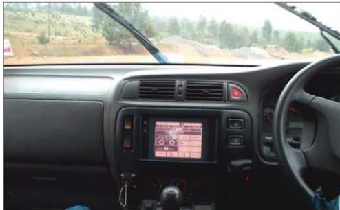
MineSuite Graphical Touch Screen mounted in shift supervisor vehicle
