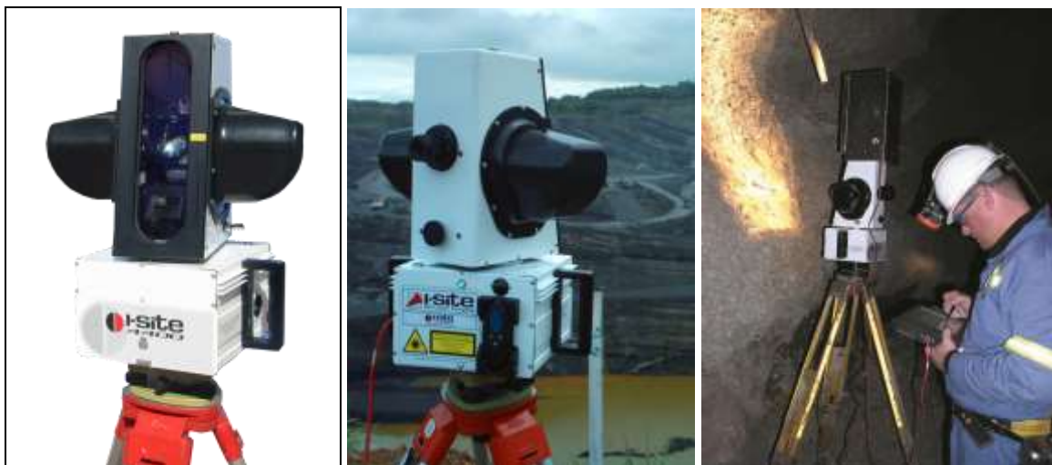
Figure 2: Front and rear view of I-SiTE scanner (left and middle) and scanner in action underground.
