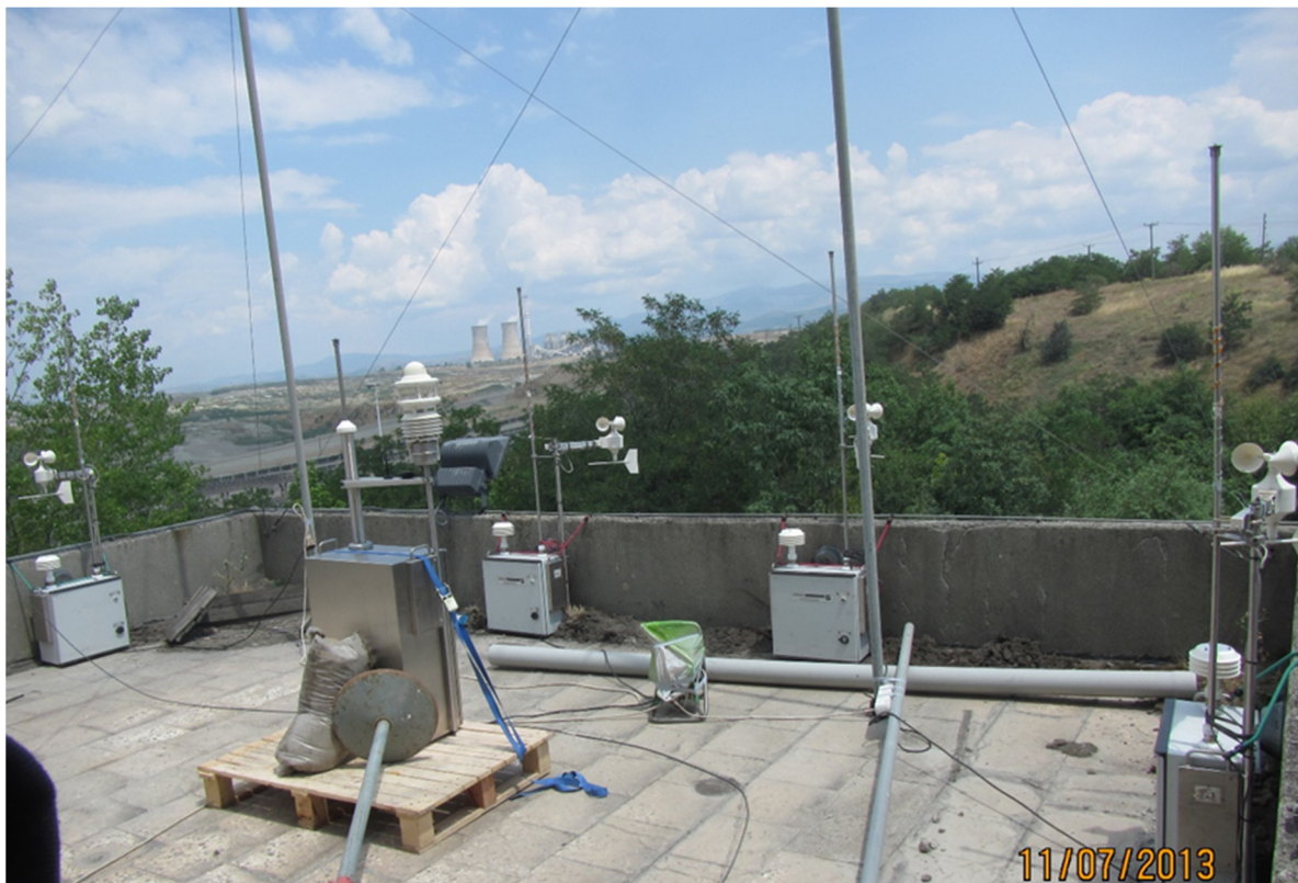
Figure 1. The five PMx monitors (Grimm) and meteorological sensors of used for the measurement campaign located on the roof of Amyntaio mine control tower. Intercomparison of equipment performed at the start of each measurement period.
