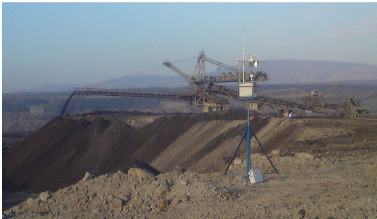
Figure 2. Stackers in the mine of Kardias field during one of the measurement campaigns. One of the installed PMx monitors is also shown.
