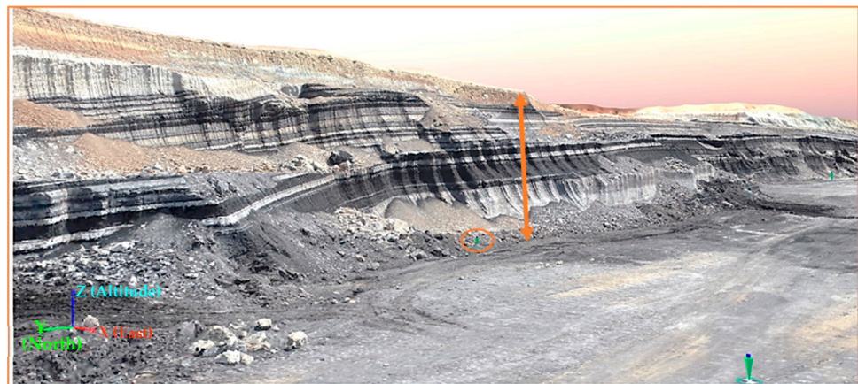
Figure 4. View of bench S3. The orange line gives the height of the front while the two green points are GCPs.
